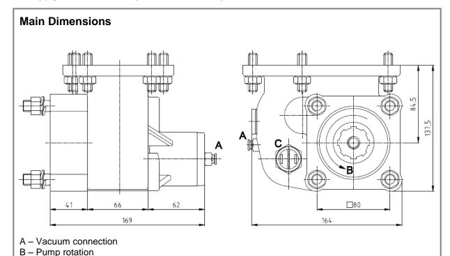
**Main Data Continuous Torque (Nm)** 150 **Intermittent Torque (Nm)** 210 Power (at 1000 rpm) 21 cv / 16 kW **Mounting Position** Left **Pump Rotation Right Hand** Weight (kg) PTO internal ratio 1:0,88 Indicative ratio from motor to PTO's output 1:0,43
