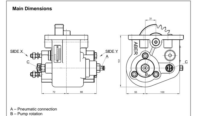
C - Option: Electric sensor with mechanical driving Ref. 18001PS
