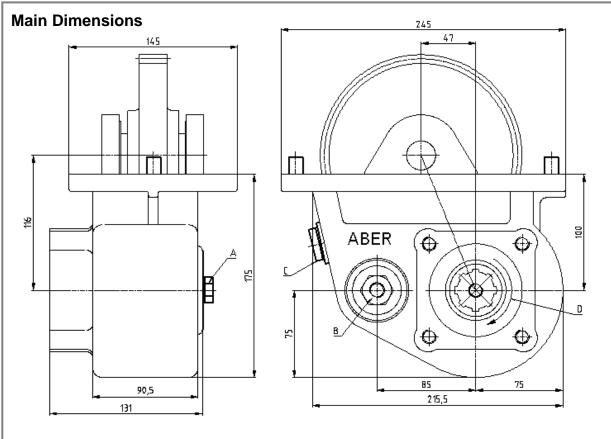
A - Option: Electric sensor with mechanical driving Ref. TF14003PS or TF14003PC
